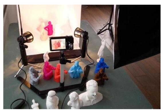
3D prints made in the studio are made using PLA plastic which comes in many vibrant colors – including sandstone, copper, gold, or silver. If customers want their 3D selfies printed in a material other than PLA, DoubleMe3d outsources to Shapeways and other 3D printing service providers.
