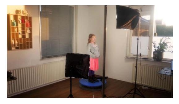
At the new 3D printing studio DoubleMe3d, customers can have their full bodies scanned. The data from these scans provides the digital geometry for making 3D printed selfies.
